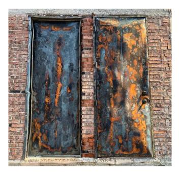
Photo 4. Details of fire door frame after hose stream test
