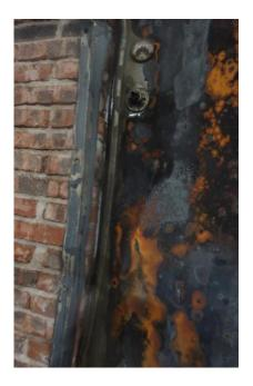
Photo 3. The strike jamb adjacent to the door latch edge of out-swing door after the hose stream test
