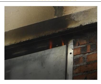
$\label{eq:Photo 1.}$  Sustained flame on top right corner of the out-swing door on 22 minutes
